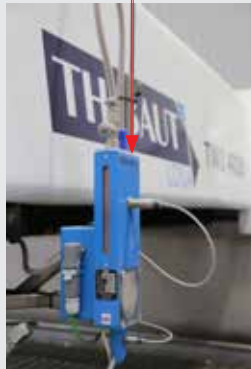
1 proportioner type Feedline V with a control unit and proportioning of the cutting head abrasive flow. Possible adjustment during the cutting.
